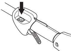
**CAUTION!** The stop switch automatically returns to the start position. In order to prevent unintentional starting, the spark plug cap must be removed from the spark plug when assembling, checking and/or performing maintenance.
