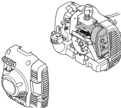
In countries that have a warm and dry climate there is a significant risk of fire. We therefore fit certain mufflers with a spark arrestor screen. Check whether the muffler on your machine is fitted with this kind of screen.
