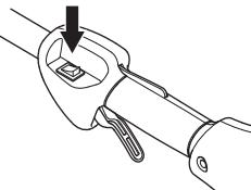
Start the engine and make sure the engine stops when you move the stop switch to the stop setting.
