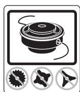
Only use non-metallic, flexible cutting attachments, i.e. trimmer heads with trimmer cord.
