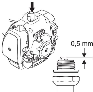
**CAUTION!** Always use the recommended spark plug type! Use of the wrong spark plug can damage the piston/cylinder. Check that the spark plug is fitted with a suppressor. Ask your dealer or Husqvarna should you need more information.
