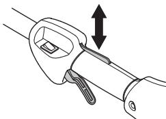
Check that the throttle trigger and throttle lockout move freely and that the return springs work properly.
