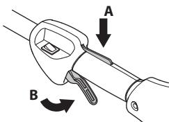
Make sure that the throttle trigger is locked at idle setting when the throttle trigger lockout is released.
