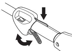
See instructions under the heading Start. Start the machine and apply full throttle. Release the throttle and check that the cutting attachment stops and remains at a standstill. If the cutting attachment rotates with the throttle in the idle position then the carburettor idle setting must be checked. See instructions under the heading Maintenance.
