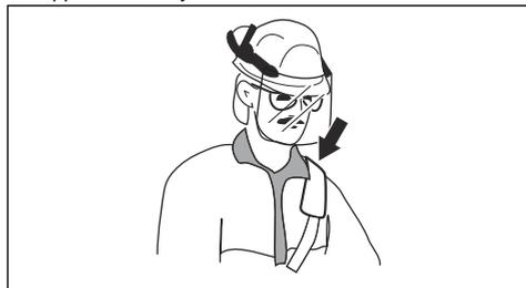
4. Adjust the harness until the cutting attachment is parallel to the ground.
