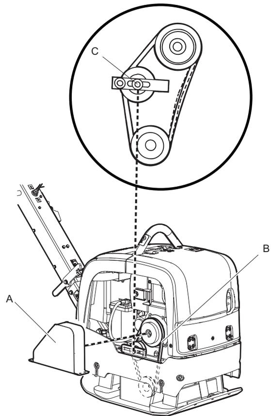
3. If the V-belt tension needs adjusting, release the belt tensioner (C) and push it backwards.
