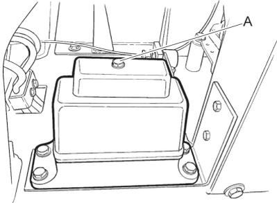
2. Fill up with hydraulic oil if necessary, see chapter "Hydraulic system, changing the hydraulic oil".
