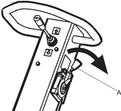
2. Set the throttle control (A) in stop position.
