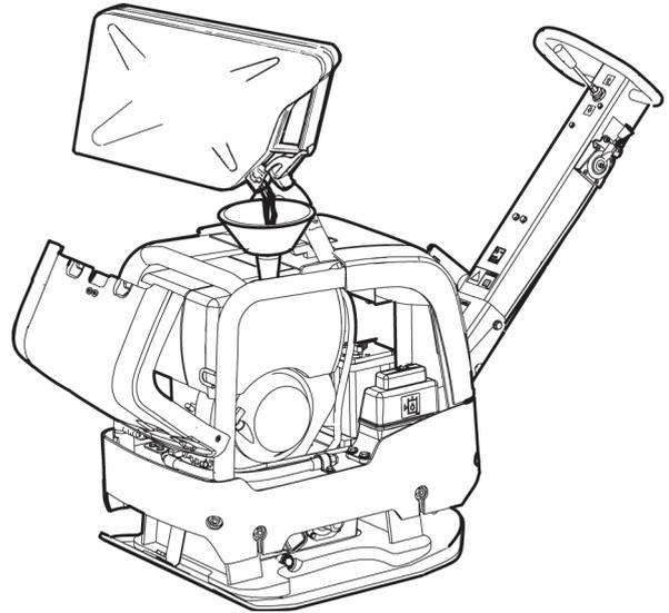
4. Never overfill the tank. Due to the movement of the fuel within the tank, it is possible to have fuel at a higher level than the tank cap, which can lead to a spillage of fuel if the tank cap is opened. This can be avoided by only opening the tank cap, when the machine is tilted and the tank cap is at the fuel tank's highest point.
