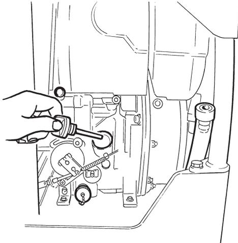
2. Set the throttle control (A) to half revs.
