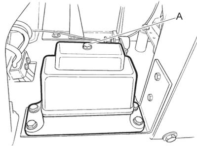
2. Use an oil suction pipe to empty the hydraulic oil from the tank.
