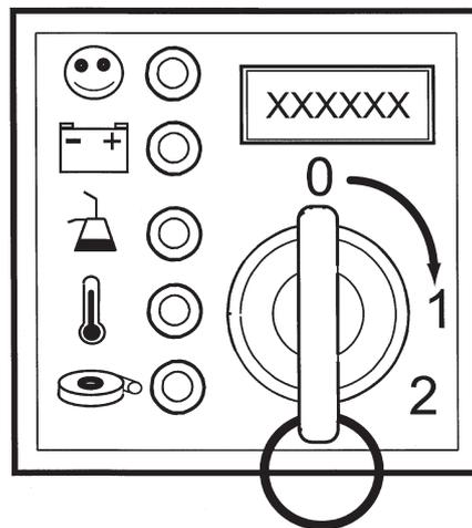
3. Turn the ignition key through position 1 to position 2.
