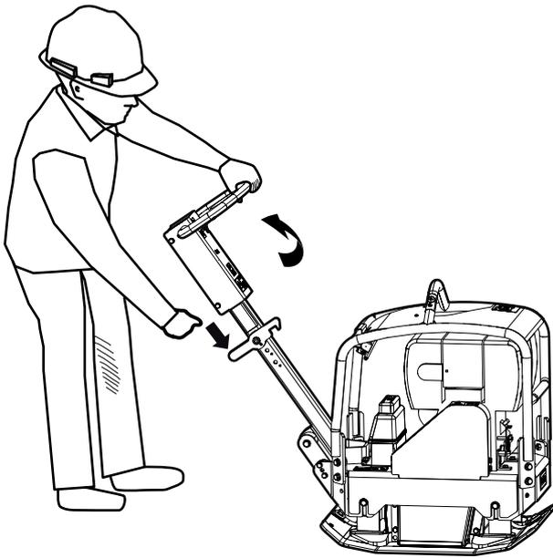
**NOTICE** During compaction work the engine must always be run at full throttle.
