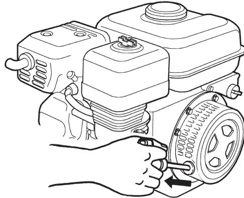
5. Move the choke valve gradually to the fully open position.
