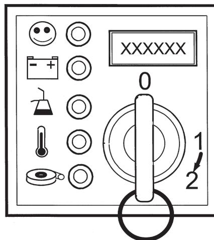
4. Release the ignition key as soon as the engine starts.
