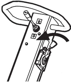
2. Close the choke valve if the engine is cold. If the engine is warm or the ambient temperature is high, close the choke valve halfway or leave it open.
