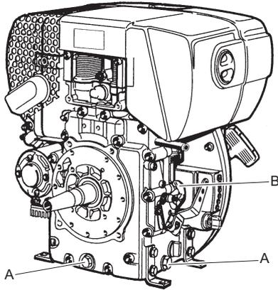
2. Tilt the machine backwards and let the oil drain in a drainage hose.
