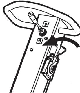
2. Turn the ignition key to ignition position 1. The control lamps for charging and oil pressure light up.
