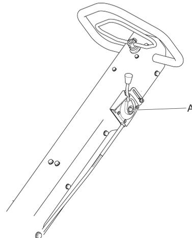
2. Lubricate the controls (A, B) if necessary.
