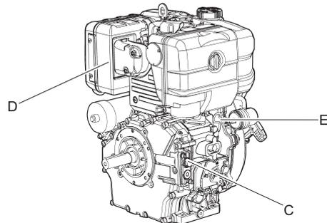
4. Fill the engine oil to the maximum mark on the dipstick (C).
