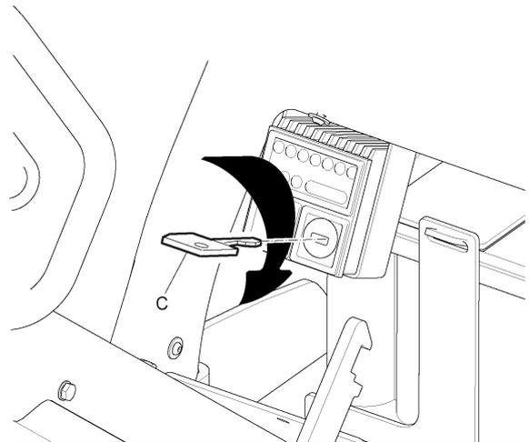
3. Turn the ignition key (C) through position II, to position III.
