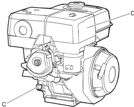
3. Loosen and refit the oil filter (C) and the air filter (D).
