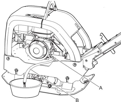
1. Open the oil drain valve (A) and drain the oil into a container using a draining hose (B).
