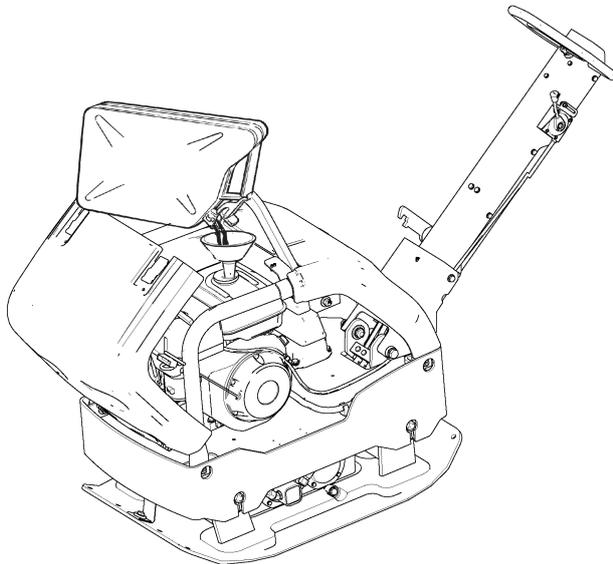
1. Check the engine oil level.
