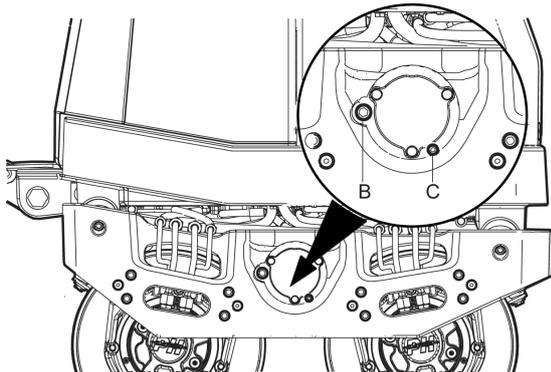
4. Remount the oil level plug (C).
