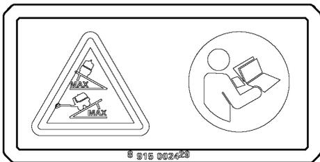
The operator must read the safety, operation and maintenance instructions before operating the machine.
