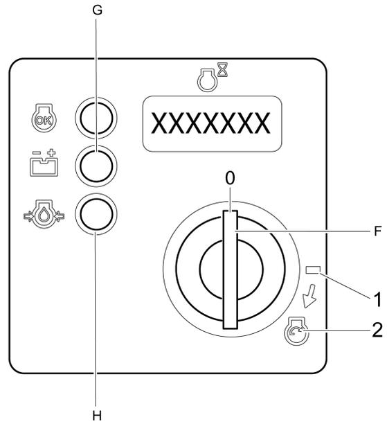
5. Turn the ignition key (F) to the starting position 2 and release the ignition key when the engine starts.
