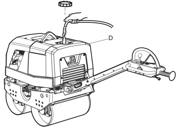
**NOTICE** During operation oil leaks can occur and bolted joints can come loose, this can cause engine breakdown.
