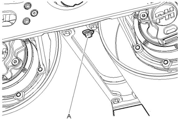
2. Drain the oil, clean and remount the drain plug (A).
