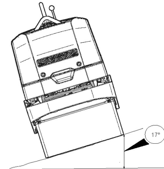
The tilting angle is measured on a hard level surface with the machine stationary. Vibration switched OFF and all tanks full.
