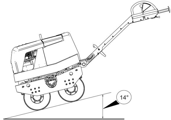
The maximum gradeability of the machine with vibration switched off is 19°.
