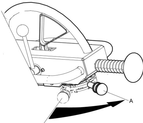
2. Turn the throttle control (B) to the stop position to stop the engine.
