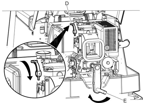
5. Turn over the engine with the starting handle (E).
