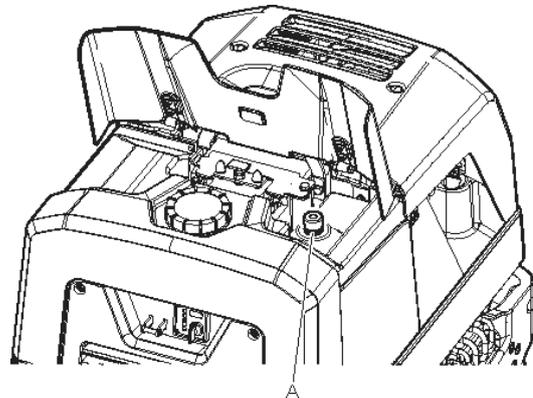
2. Use an oil suction tool to empty the hydraulic oil from the tank.
