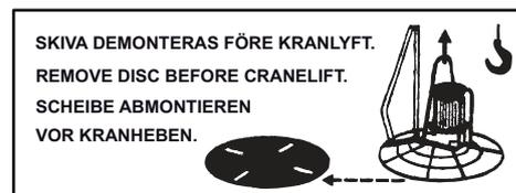
◆ Remove disc before crane lift.
