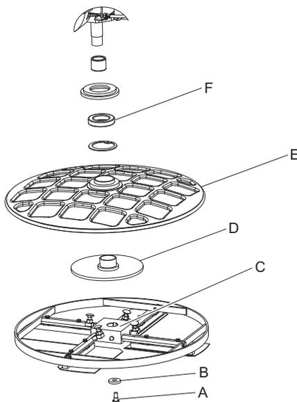
2. Dismount the spider assembly (C). Use a puller if the blade cross is tight on the shaft.
