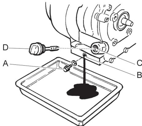
2. Tilt the machine backwards and let the oil drain in a drainage hose.
