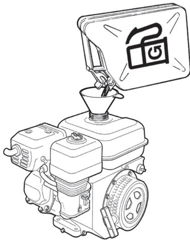
4. Never overfill the tank. Due to the movement of the fuel within the tank, it is possible to have fuel at a higher level than the tank cap, which can lead to a spillage of fuel if the tank cap is opened. This can be avoided by only opening the tank cap when the machine is on level ground and the tank cap is at the fuel tank's highest point.
